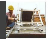
Release the support frame and swing out towards the eves of the roof. Engage the hooks so that the frame is angled towards the eves and not under the platform.
